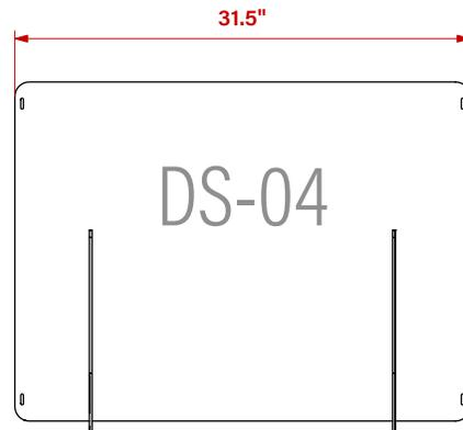
Shield made of optically clear  $\frac{1}{8}$ " polycarbonate.
