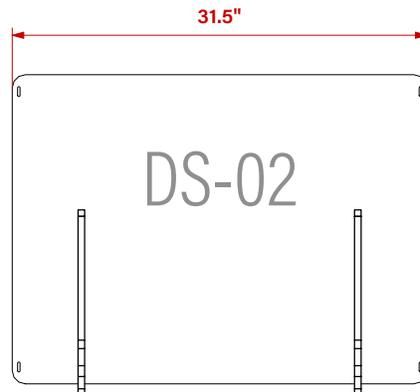
Shield made of optically clear  $\frac{3}{16}$ " polycarbonate.
